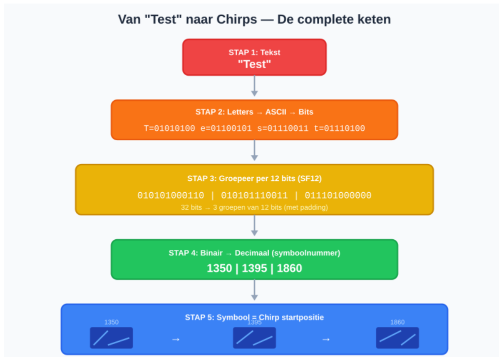
Figure 3: From "Test" to chirps — the complete encoding chain
